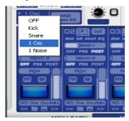
Assign to the first three sound generators the "1 Osc" randomizer. Make sure that the three bands are set to be triggered by the three notes you used to compose the random sequence.
